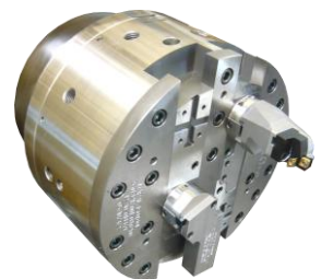
Facing head with 2 numerically controlled slides; mechanical interfaces for application-specific tool holders and (optionally) counterweights
